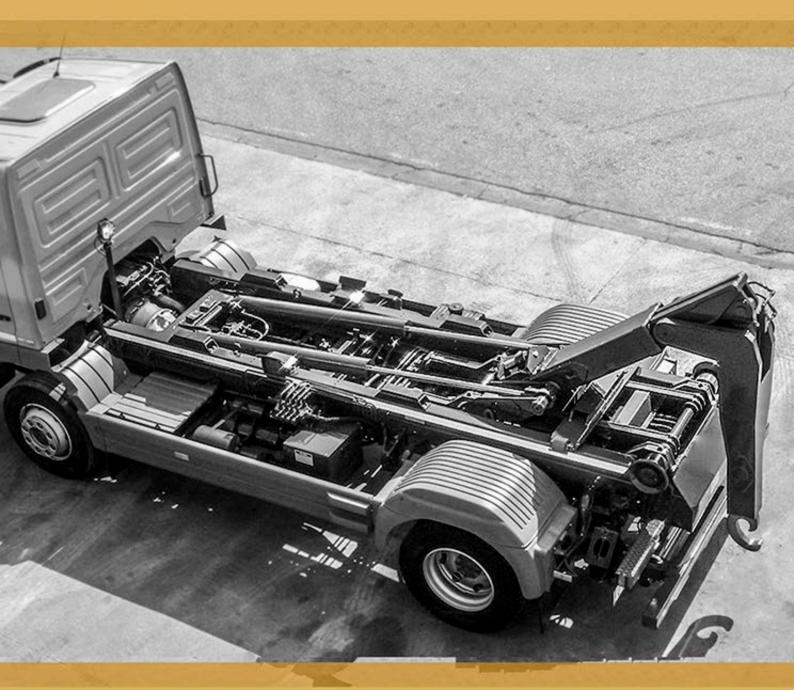
ELS hooklifts have a lifting capacity from 3TN. to 30TN. They all are internationally tested in the most demanding fields, allowing for the safest and most reliable transport of containers.
