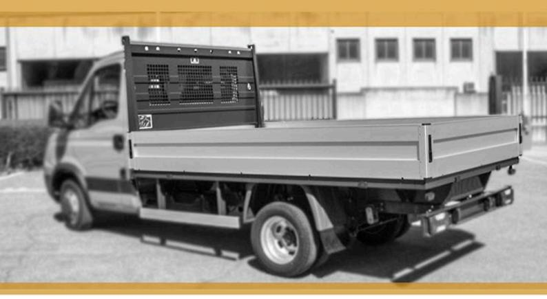
Sidewalls are composed by steel sheets in different heights, which are foldable and removable.
