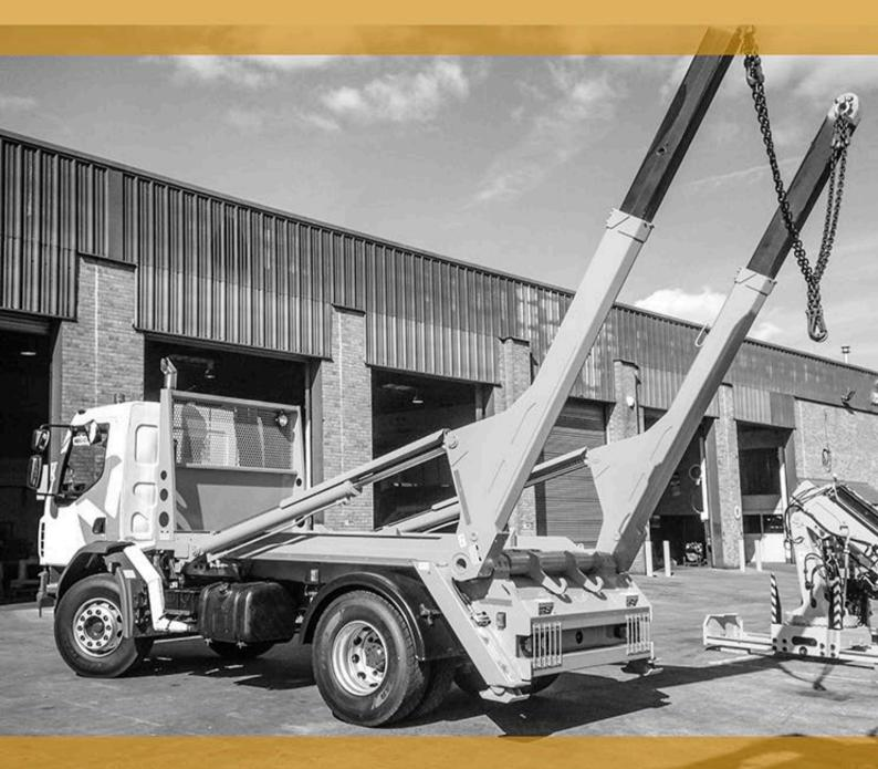
Durability typifies our equipments. We have a wide range with lifting capacity from 3TN. to 18TN. They are also equipped with robust hydraulic telescopic arms and independent drive rear support feet. Standard equipment includes pneumatically activated DIN type balancing hooks. Wide range of optional elements is available, including cargo containers.
